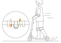
4. Slow down by releasing the throttle. Squeeze the electronic brake and stamp the rear fender with foot at the same time for a sudden brake.
