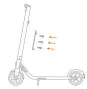
Install the external battery on the rail and fix it with the M4 (20mm)
