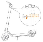
Firmly connect the wires inside the handlebar and the stem. Slide the handlebar onto the stem. Be aware of the correct orientation.
